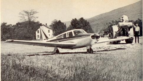
One reason for the increased performance of the Comanche 260 is the single-fork main landing gear strut, which when retracted greatly reduces drag. A feature of the 260 is the very short main landing gear strut with full travel oleo shock absorber
